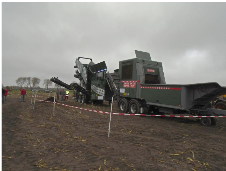
Figure 13: Ballistic separator used to purify biomasses
