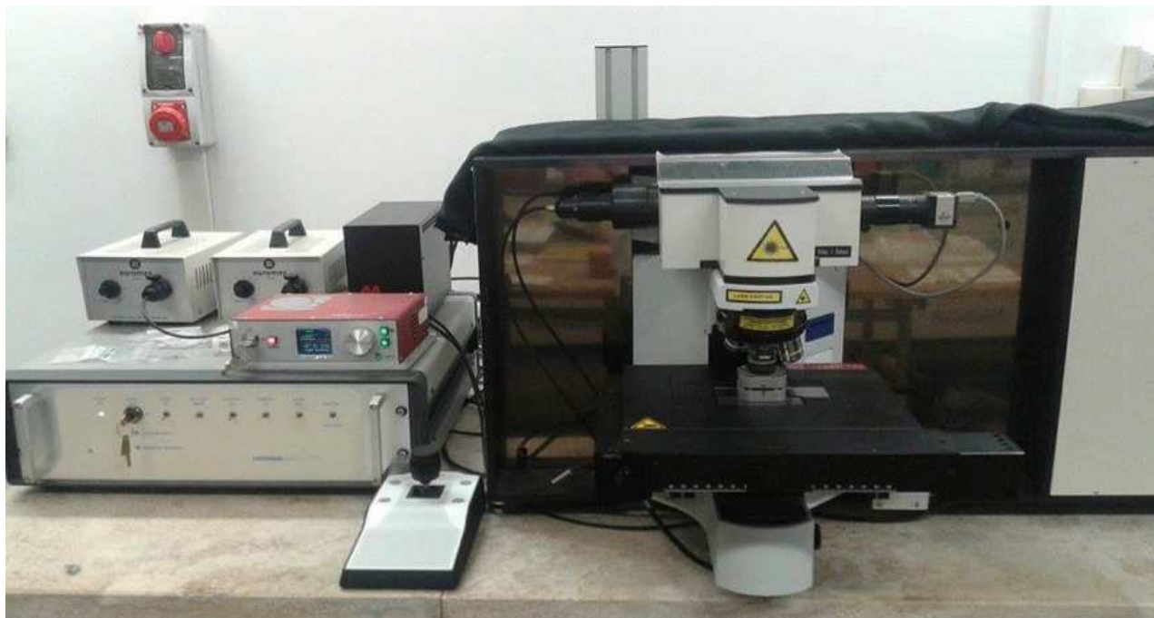
Figure 2.7: Horiba LabRam HR micro-Raman spectrometer (Department of Sciences, University of Roma Tre).
