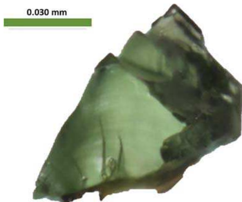
FIG. 1. The single crystal of jeffbenite studied in this work on which the crystal structure was determined together with all further physical and optical properties. The emerald green colour is characteristic for this phase.
