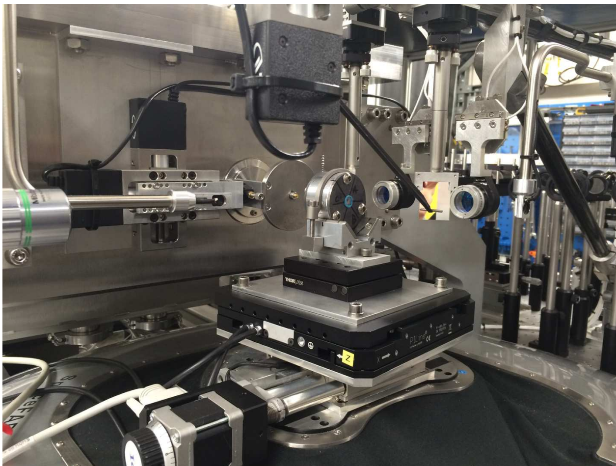
Figure 2.11: Synchrotron X-ray powder diffractometer (Diamond Light Source, Rutherford Appleton Laboratory, United Kingdom).
