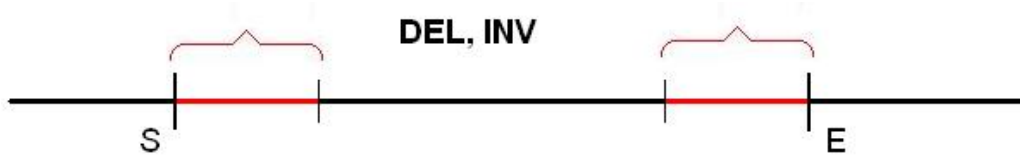
Figure 2.11: In case of deletions or inversions longer than 6 * StdDev (so E - S > 6 * StdDev ), reads are splice-aligned only on red positions; if E - S \leq 6 * StdDev , reads are splice-aligned in all positions between S and E .
