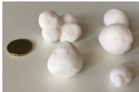
Figure 2.7: Ball growth of and over-granulation of the formulation containing 100% (w/w) of sorbitol.
