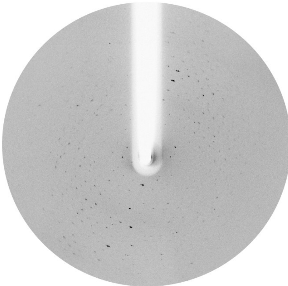
Figure 3.4 Detail of the diffraction image collected at the European Synchrotron Radiation Facility beamline ID23-2 gemini (ESRF Grenoble, France); the external spots correspond to a maximum resolution of 8 Å.
