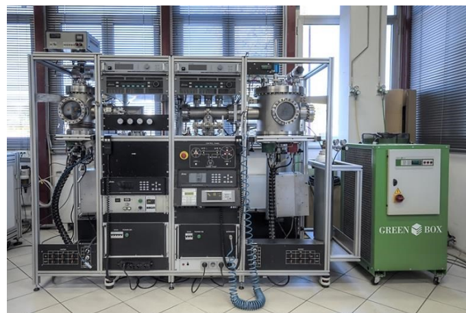
Fig. 7.1: magnetron sputtering machine. The chamber used for the depositions is the one on the left.
