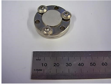
Fig. 9.15: stainless steel HiPIMS sample holder with a sample after the sputtering process. Screws fasten the sample and guarantee electrical contact.
