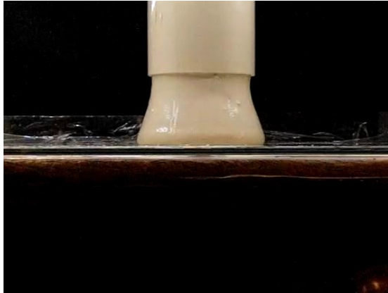
Figure 7.1.3 Initial release of the material for the WK1 big cylinder test ( t=0.30s ).
