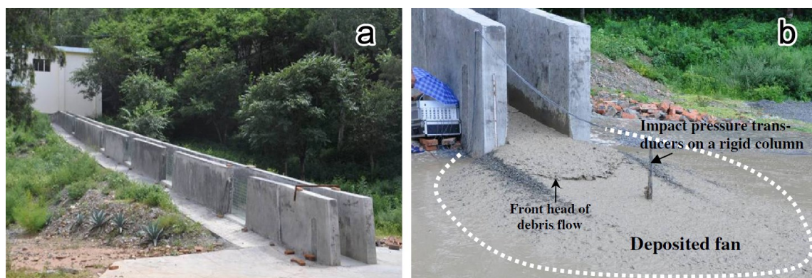
Figure 5.3.2 Flume apparatus used by Zhou et al. (a) Picture of the experimental setup. (b) Entrainment of bed materials and formation of downstream debris-flow surges.
