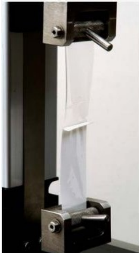
Figure 3.1: Example of a tensile strength test of sealed polymeric material. The test measures the force necessary to open the seal tearing apart the extremities of the stripe.
