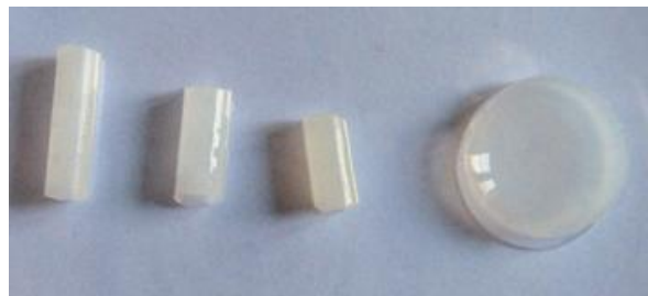
Fig. 4. Tubular (diameter 2 mm) and disk-shaped (diameter 15mm) scaffold.
