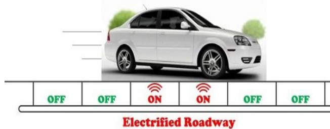
Fig. 2.3. WPT track and its segmentation.
