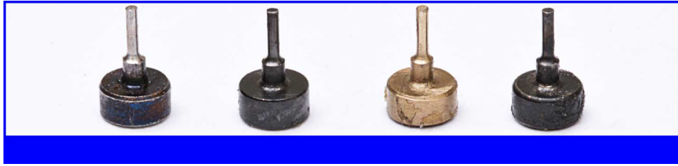
Figure 6.5: Coated mold insert used for the characterization of the ejection force.
