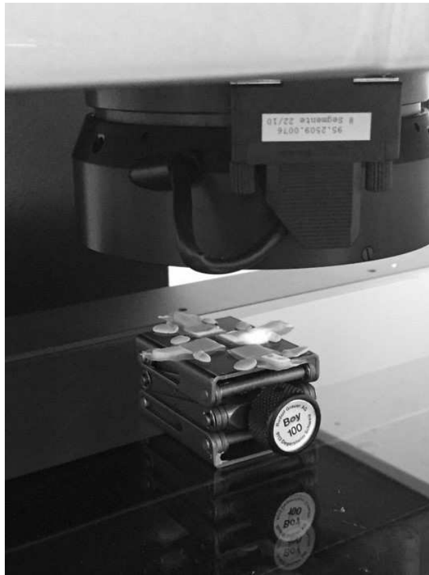
Figure 14.5: Measurements of the molded parts with the CMM machine.
