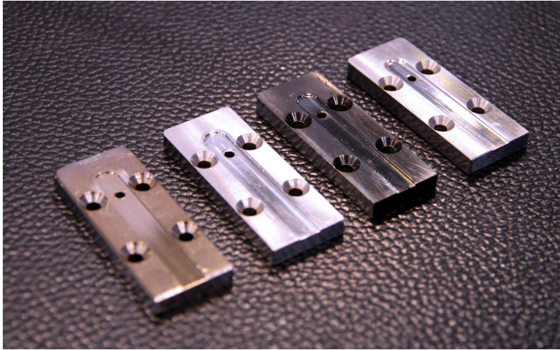
Figure 6.4: Coated mold insert used for the characterization of the melt flow resistance.
