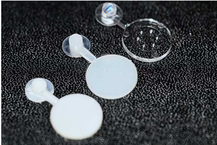
Figure 12.4: Injection molded parts with the three different polymers.
