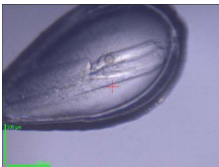
Figure 3.7. An example of 20S proteasome crystal properly mounted in a loop for X-Ray diffraction data acquisition.
