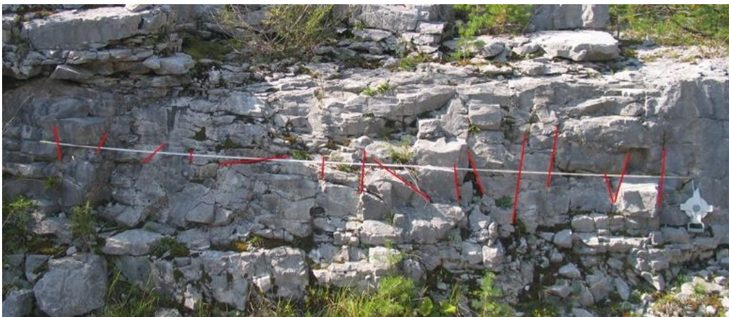
Figure 4. 3 – Typical example of joints system (red segments) intersecting a scanline. The tape length is almost 3m.
