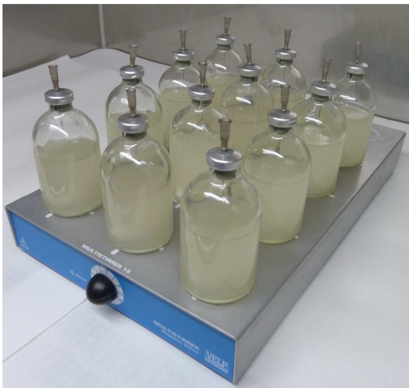
Figure 2.1 – Experimental setup for yeast fermentation in 120 mL serum bottles on magnetic stirrer.
