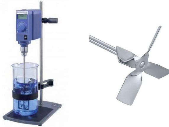
Figure1. 5: Overhead stirrer (left) and rod (right) used for the production of geopolymers.
