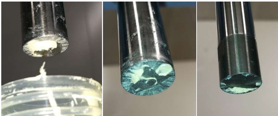
Figure B.8: Adhesion loss with the geopolymeric slurry after 56 minutes
