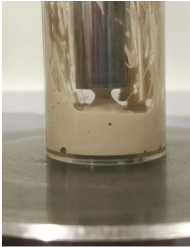
Figure B.3: Deformation of the pulled geopolymer cylinder
