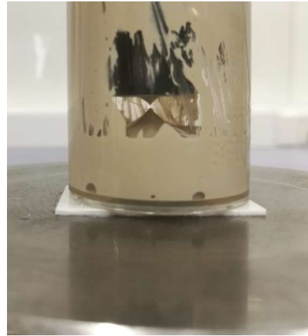
Figure B.4: Geopolymer cylinder detachment
