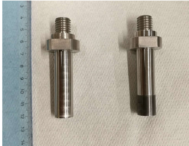
Figure B.1: Steel (left) and WC (right) probes used for tack tests
