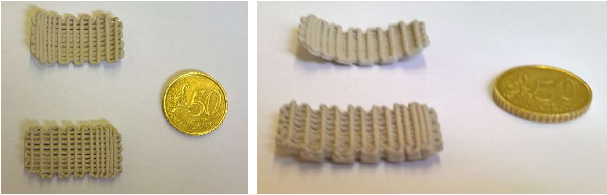
Figure 2.1: Samples printed with PEG 400 5% wt. and water ratio = 14.0; sample above is printed before the one below.
