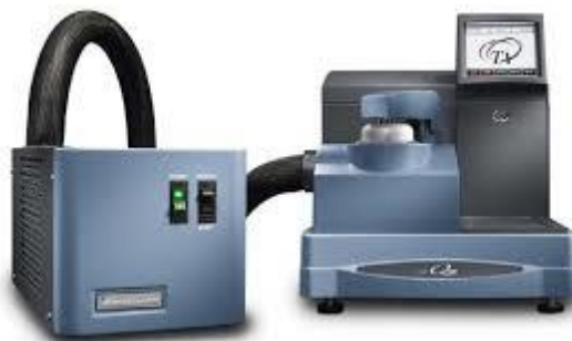
Figure 2.19– Differential scanning calorimetry (DSC Q200)
