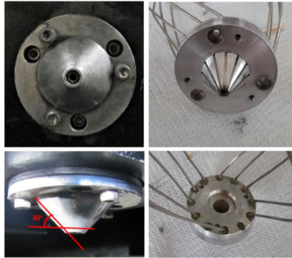
Figure 2.5- Coaxial nozzle used for powder injection in MSL50 machine, Manudirect
