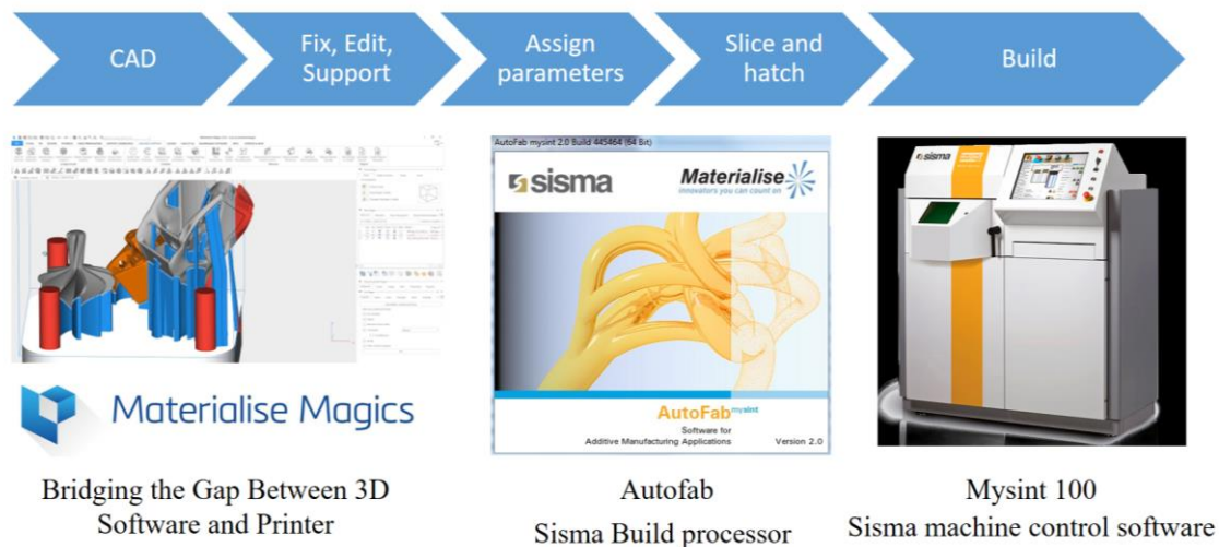
Figure 2.17– Roadmap in SLM process
