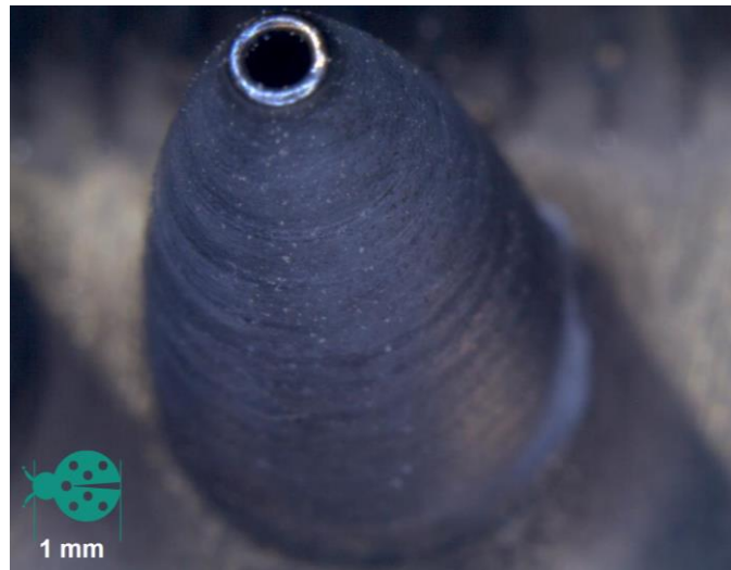
Figure 3.46– Ti-Al-Nb cone produced by \mu DMD using heat decay model (in collaboration with Manudirect company)
