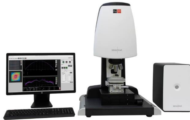
Figure 2.22– Optical profilometer (Sensofar Plu Neox)
