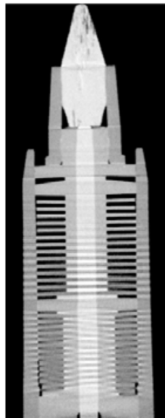
Figure 5.5: Example of cone-beam artifact in circular scanning trajectories. As visible in the upper and lower part of the image severe cone-beam artifacts are present on flat surfaces [112].
