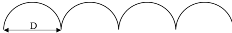
Figure 6.12: Theoretical FDM profile. Ideally a periodic profile is generated with period equal to the diameter D of the extruded wire.
