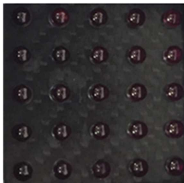
Figure 4.40: Calibrated ball plate used for the experimental investigation.
