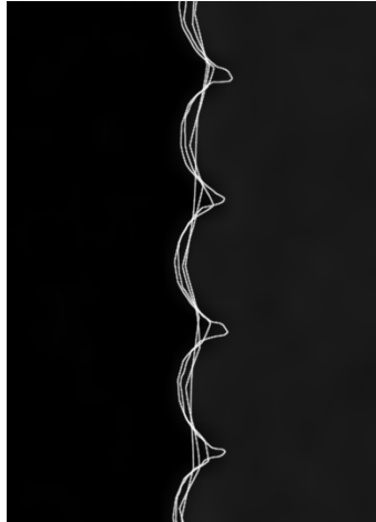
Figure 6.29: Detail of a CT section of the FDM sample. The same surface profile obtained from the CT scans performed with the four different voxel sizes is represented, after the surface determination step and alignment of the CT volumes.
