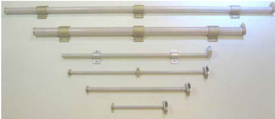
Figure 3.3: Magnetic torquers of different lengths for space applications. Photo courtesy of Cayuga Astronautics.
