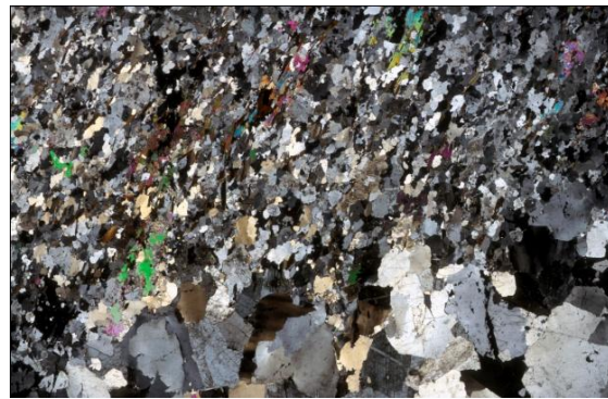
(D1) Contact between two mica orthogneiss and border zone of the pegmatite. An equigranular development of K-feldspar and quartz with subordinate polysynthetic plagioclase are observable.
