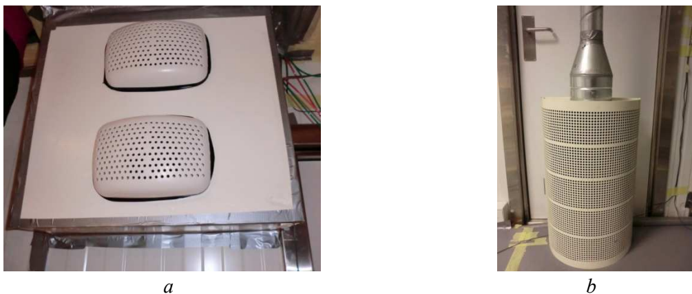
Figure 8. 6 Wall mounted supply (up) and extract (down) air terminals for mixing ventilation (a) and displacement ventilation terminal (b) in the test room
