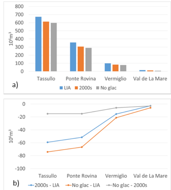
Figure 62: Scale effect on the annual runoff from 1940 to 1951 ( 10^6 m^3 ). The second panel represents the difference.
