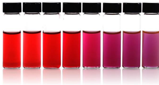
Figure 1.2 - Gold nanoparticles in aqueous solution. The red colour of the solution is linked to the SPA, and the variations are linked to the dimensions of the nanoparticles.
