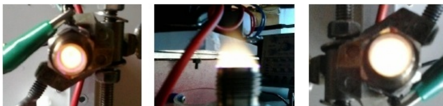
FIGURE 5.4: N_2O gliding arc reactor in operation.
