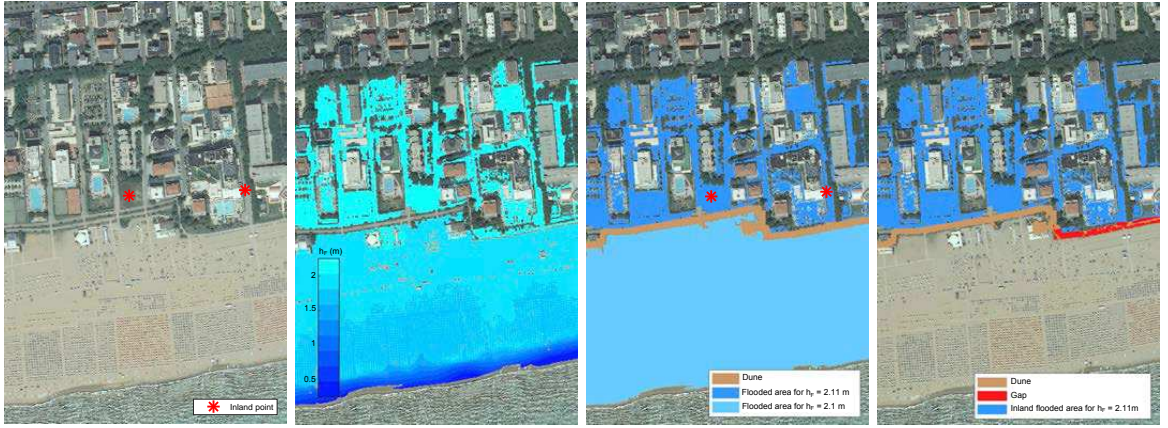
Figure 4.6: Dune and gap detection, from left to right: 1) inland control point, 2) flooded areas for different values of flooding height h_F , 3) Detection of dune, 4) Detection of gap
