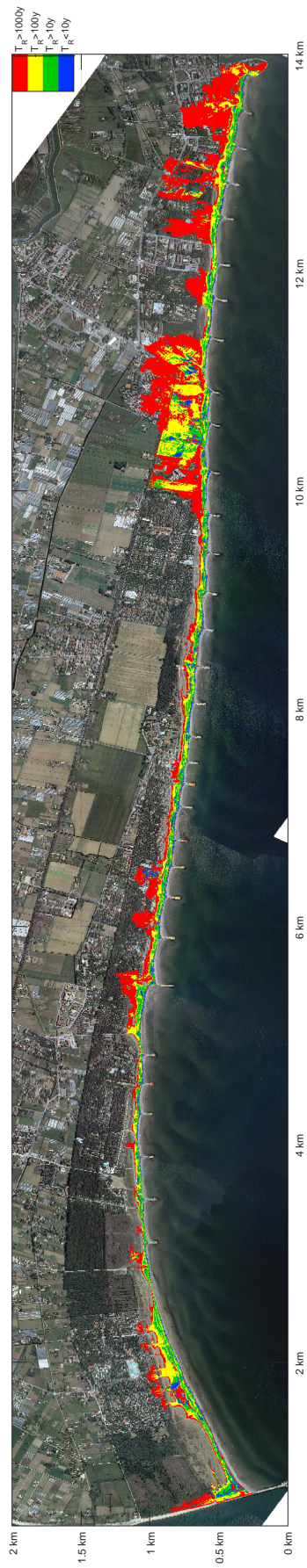
Figure 6.50: Present hazard map (cell VE6): Probability that flooding level 0.2 m is exceeded, expressed as return period T_R
