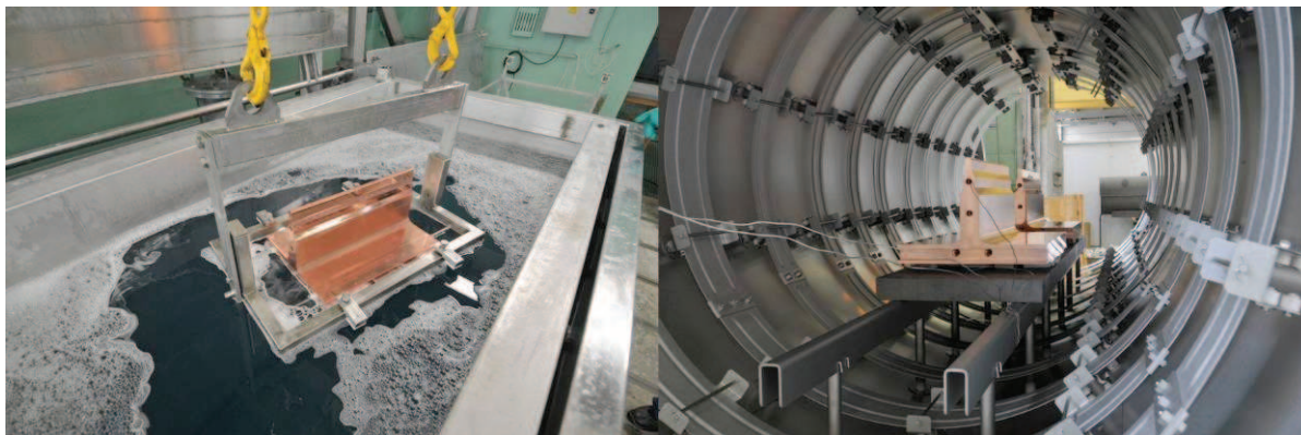
Fig. 6: Chemical degreasing and annealing process performed at 800^\circ C in vacuum condition.
