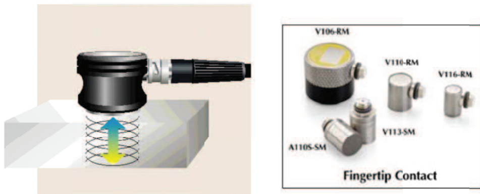
Figure 3.62 General operating conditions of a contact transducer (left) and different types of contact transducers (right) [31]
