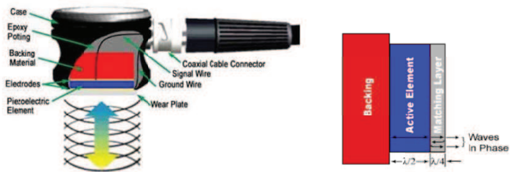
Figure 3.58 General structure of an ultrasonic transducer [32]
