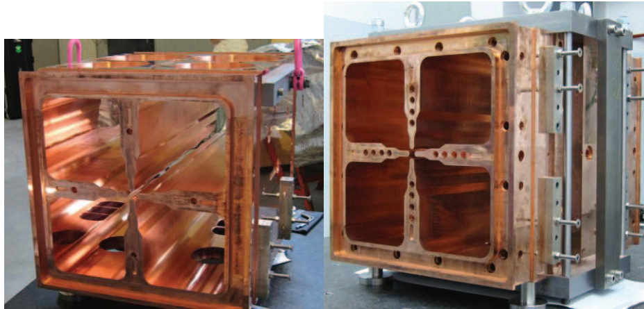
Figure 5.24 Dry assembly construction (left) and the cavity locked by the tool after the alignment of the electrodes (right).
