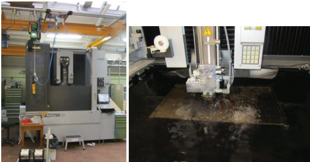
Figure 5.3 Overall view of the EDM in the INFN of Padova mechanical workshop (left) and the EDM during the EDM cut of an electrode from a copper block (right)
