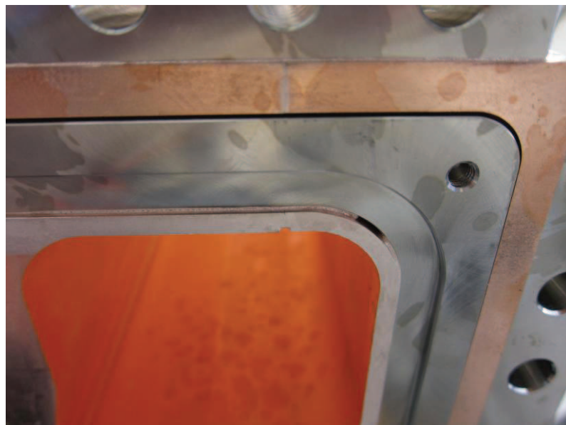
Figure 4.17 Detail of the copper-steel frame brazing on the miniprototypes brazed at LNL
