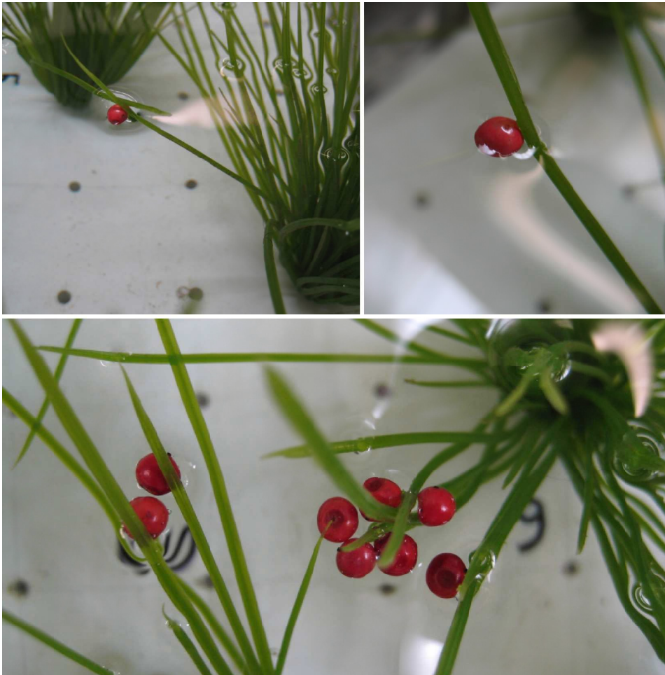
Figure 2.1: trapping of floating berries (particles B ) by emergent vegetation: examples of net trapping capture and capture by the Cheerios effect.
