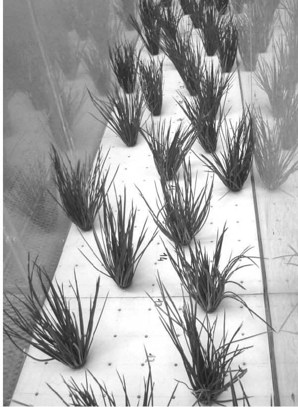
Figure 2.3: Overall view of the flume with plastic plants used in the experiments: n_p = 55.6 plants/m 2 , random pattern.
