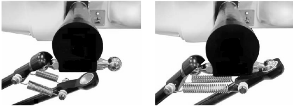
Fig. 5.4 Installing ball joints.
