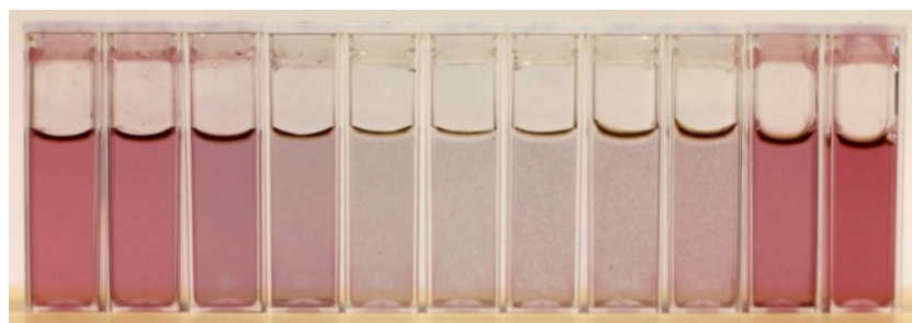
Figure 23 – Data (top) and picture of the cuvettes (bottom) from crosslinking experiment on biotinylated nanoparticles (89% ZW / 11% Biot-6). Wavelength corresponding to the plasmonic maximum (squares) and its absorbance (circles) are shown. Avidin equivalents calculated taking into account 18% biotin availability on the nanoparticle surface.
