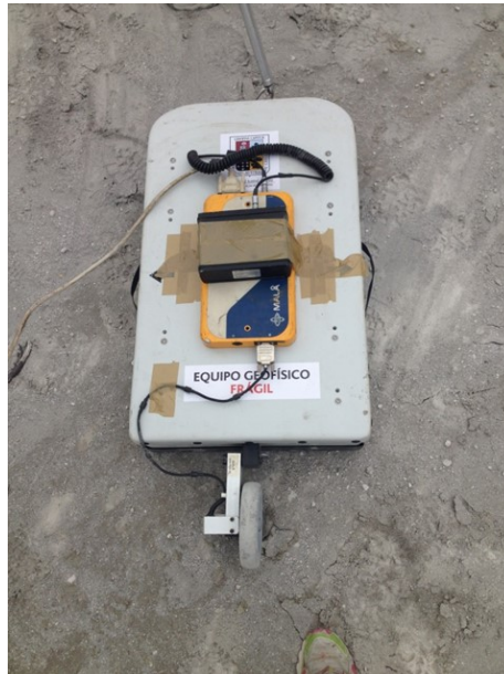
Figure 27: the GPR MALA RAMAC X3M used in this study.
