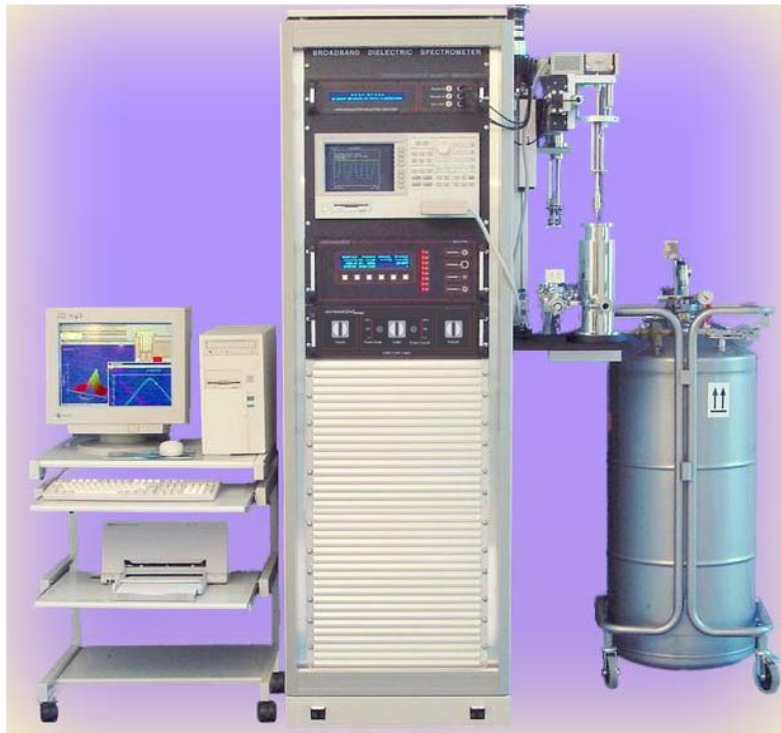
Figure 3.6. BES measuring system including the analyzer, temperature control system, the cryostat, the sample holder cell, and the vacuum pump (hidden), and electronic data management.
