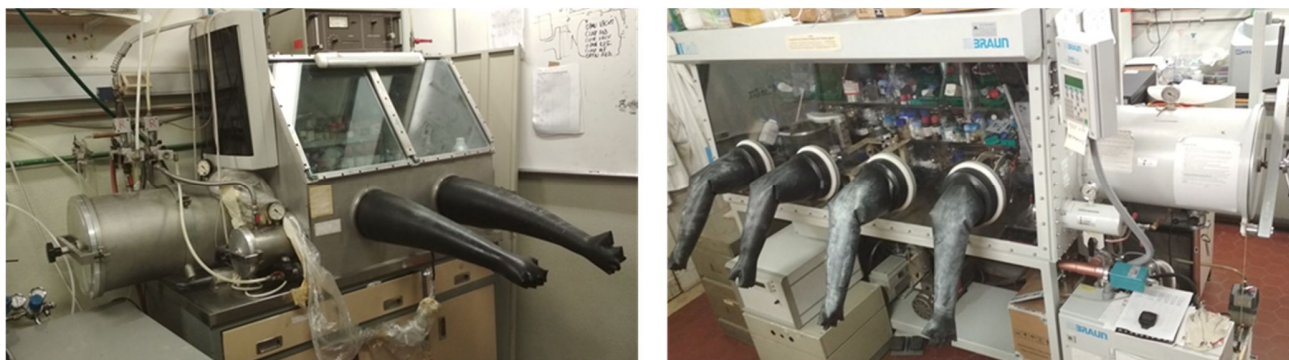
Figure 3.1. Dry- box used: homemade on the left and commercial model on the right.
