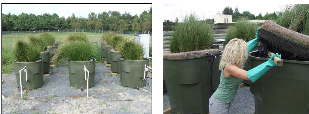
Figure 1: Floating treatment wetland experiment set up and a detail of the floating mat and roots coming out from it.
