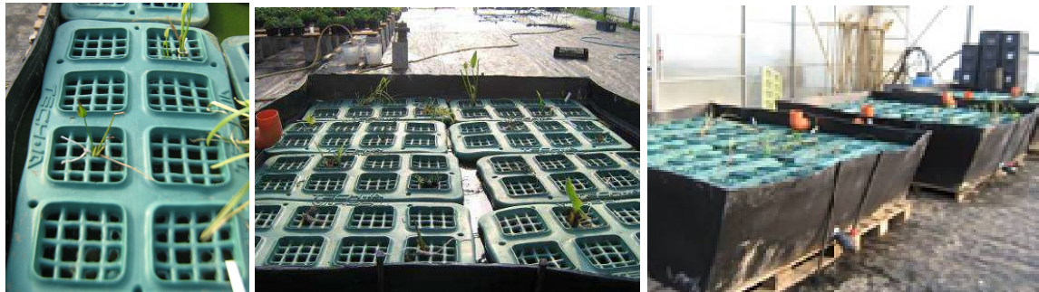
Figure 1: Tech-IA floating system used in the experiment. On the right side a single element, in the middle a basin with eight pieces and on the left the experimental set up with three repetitions.
