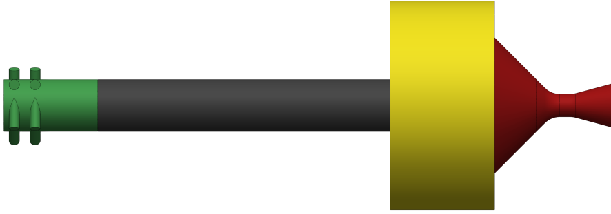
Figure 4.7: Flow field associated with the hybrid motor and divided by color into injector, fuel grain, post-combustion chamber and nozzle
