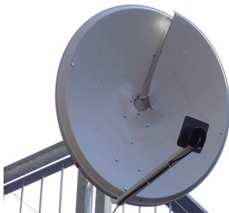
Figure 1.5: A conformal off axis parabolic reflector. Source: [56].
