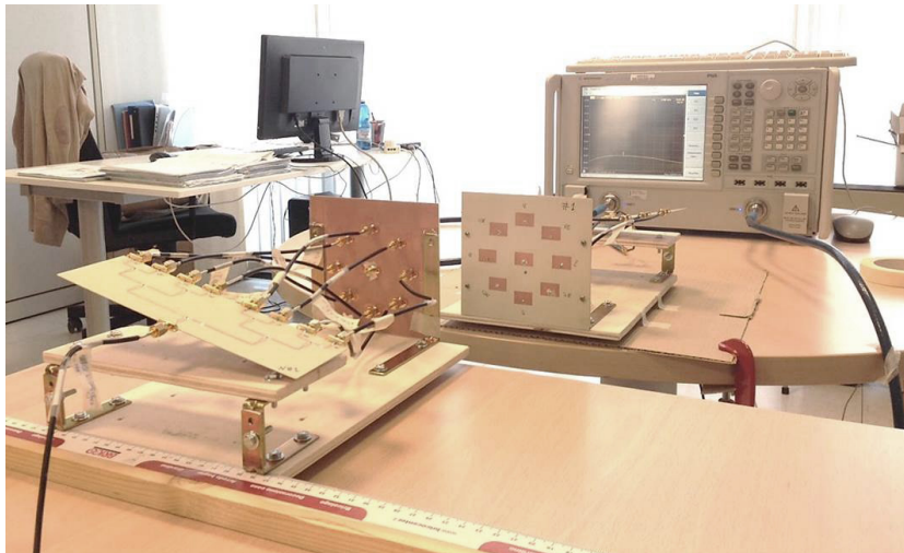
Figure 8.11: Experimental setup for the evaluation of the tolerance with respect to a lateral shift of the Tx array. The ruler, used to measure the translation shift, is visible on the bottom side.
