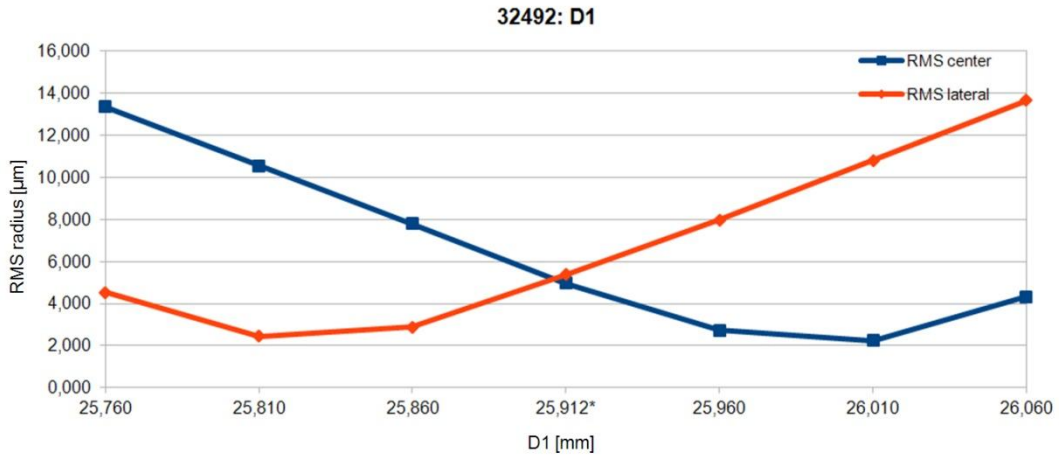
Figure 3-14 Spot RMS radius versus CCD-lens 1 (D1) distance variation for the commercial lens set configuration.
