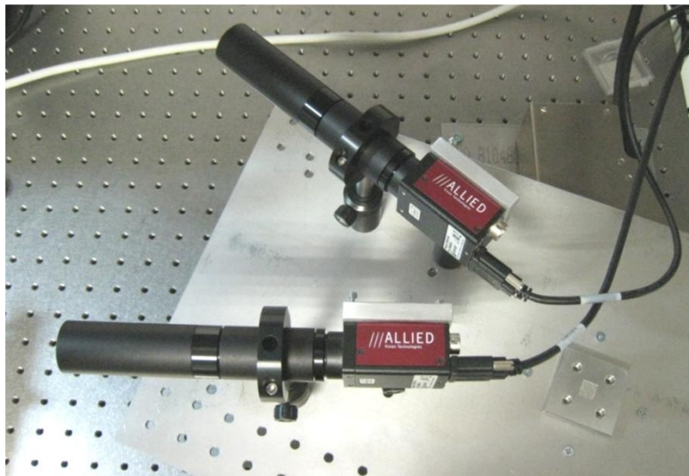
Figure 3-27: Stingray F-033B monochromatic cameras mounted over the STC FB rotating support plate with custom optics lens assembly.
