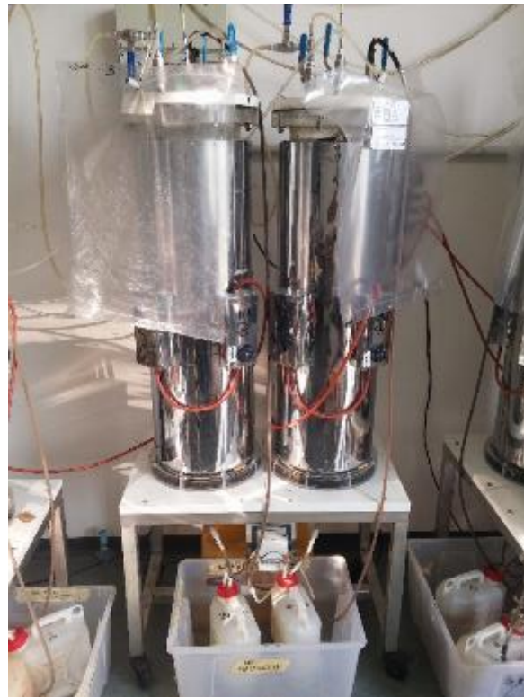
Figure 1.3.3: Picture of columnar reactor equipment with Tedlar bags for biogas collection and leachate recirculation system.
