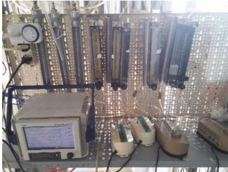
Figure 1.3.5: Particular of the air injection pumps and flow meters. The temperature monitoring equipment is visible on the bottom left side of the picture.
