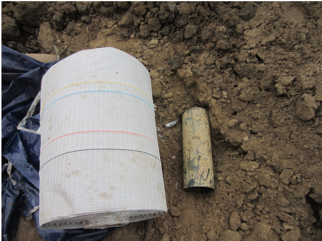
FIGURE A.13: Distributed temperature and strain sensors: 4 optical fibres encased in a 33 cm wide geotextile strip.
