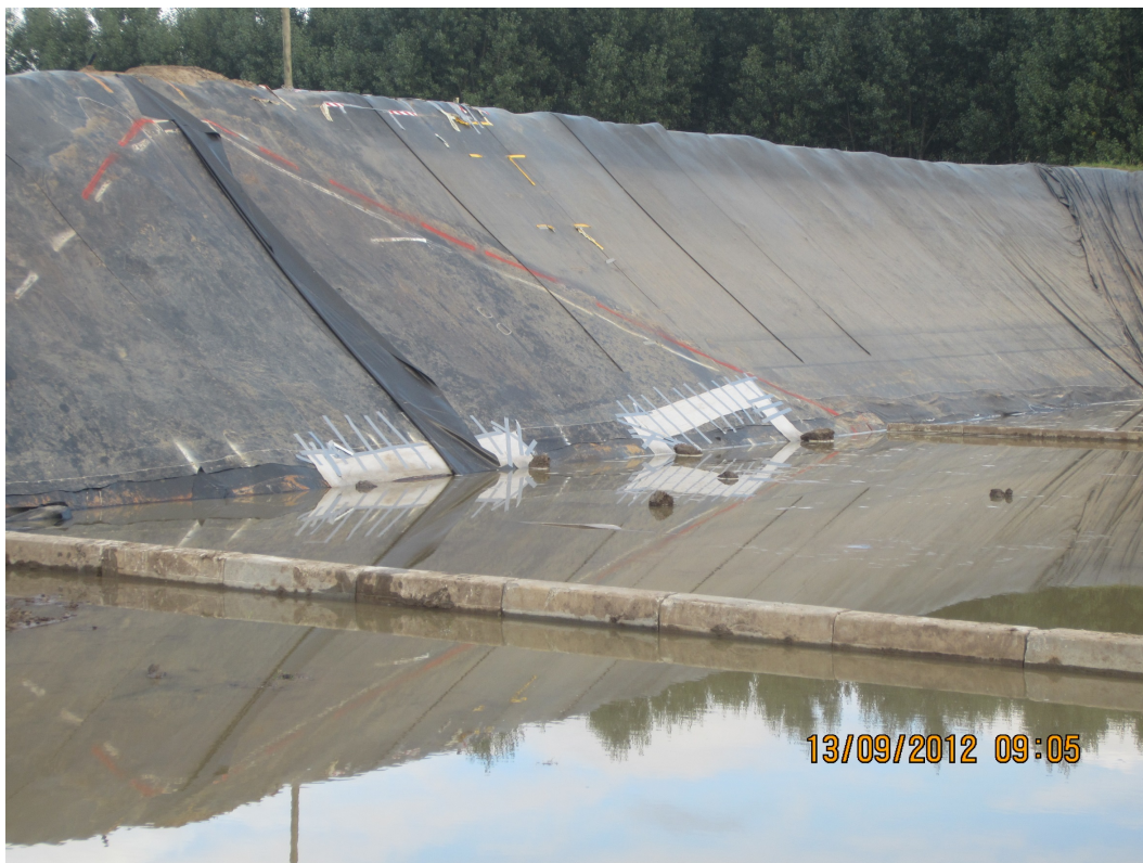
FIGURE A.15: Detail of the optical fibres at the base of the dike: bending between two profiles.
