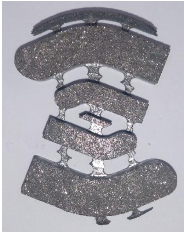
Fig. 82 – The final shape of compression self-prepared magnets
