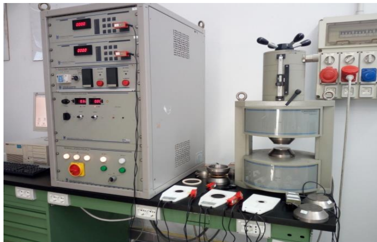
Fig. 24 - Hysteresisgraph: measurement system used for obtaining demagnetization curves
