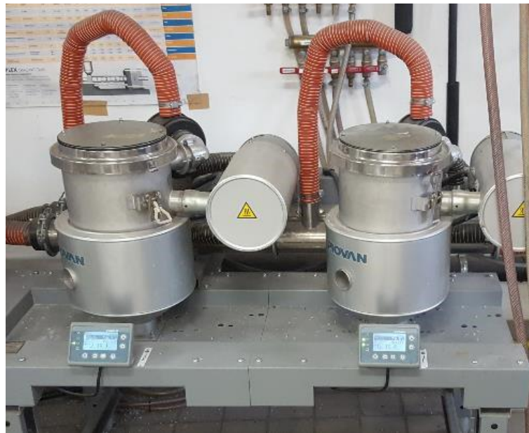
Fig. 87 – The dryer system used for about 4 hours at temperature of 80°C
