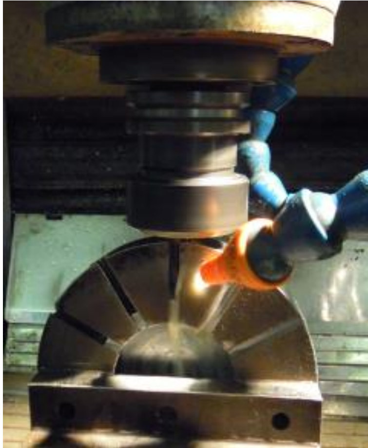
Fig. 148 - The machining of a single disk, the preparation of the stator slots
