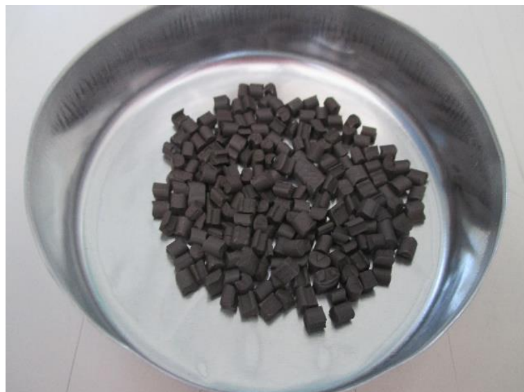
Fig. 64 - Commercial ferrite pellets used in injection process
