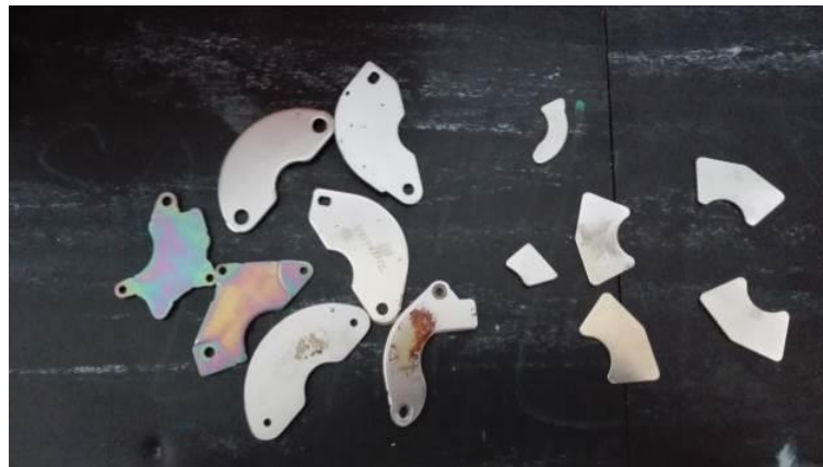
Fig. 40 – Various recovered magnets after the demagnetization process
