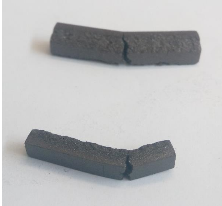
Fig. 93 – Failed insert of flexible magnets
