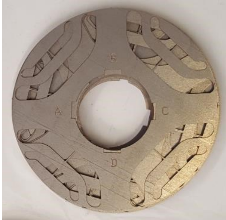
Fig. 99 – Electrical sheets/laminated steel with the flux barriers
