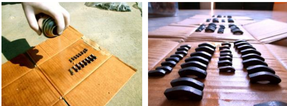
Fig. 90 – Magnets surface protection applying a protective spray
