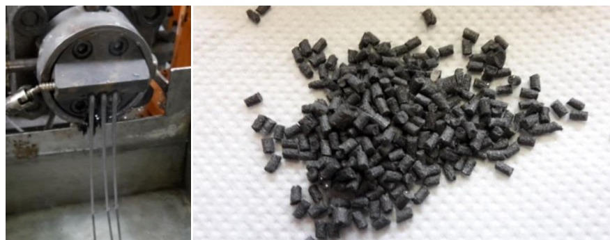
Fig. 34 - Pellet production: the case of PA6 NdFeB (self-prepared 20%)
