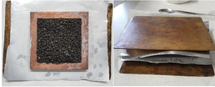
Fig. 83 – Filling of the mold with the pellets
