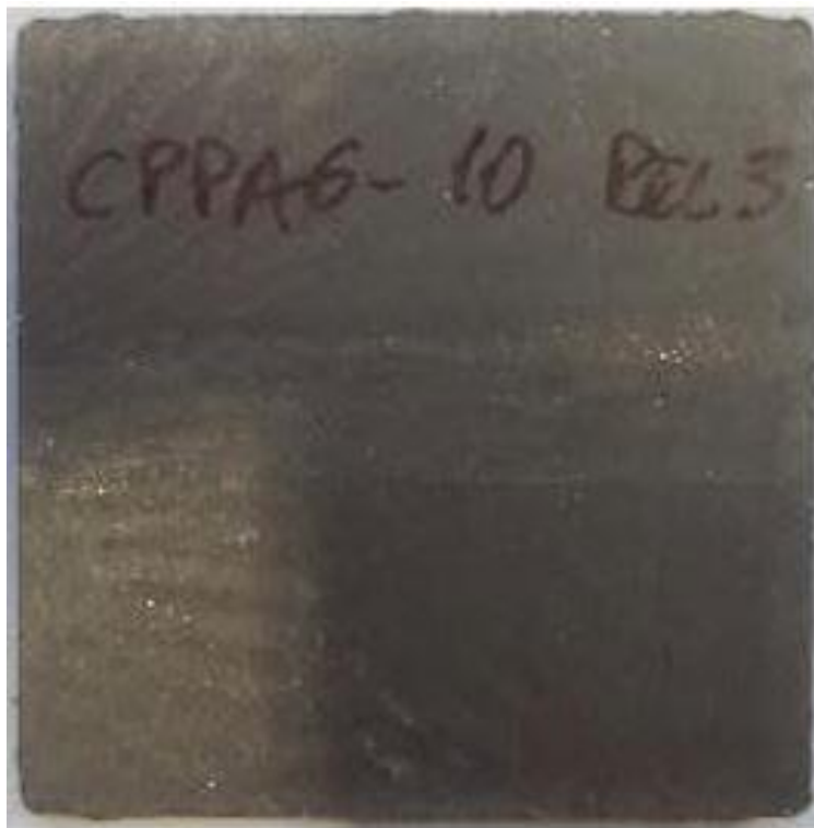
Fig. 92 - The molded sample of self-prepared PA6 NdFeB Bonded magnets
