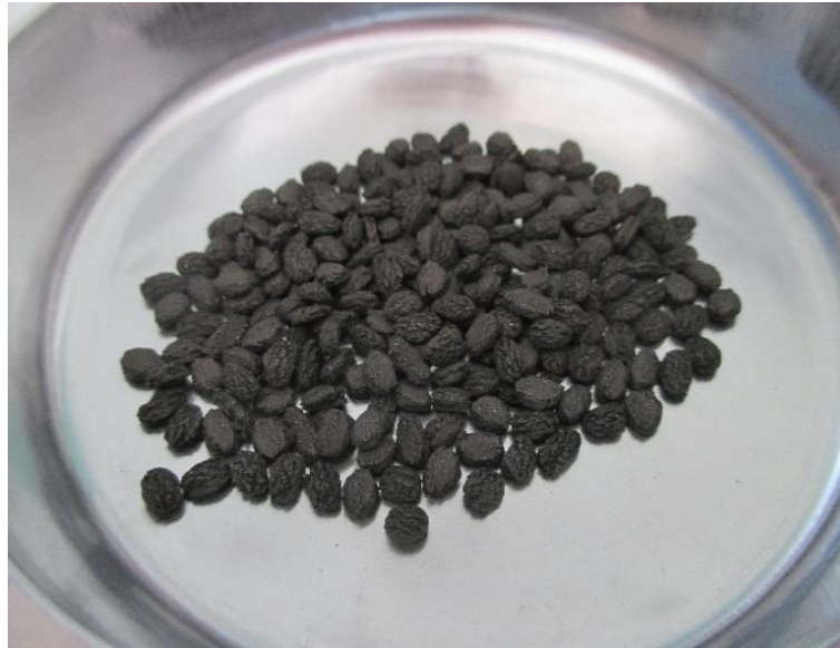
Fig. 62 – Commercial NdFeB pellets used in injection process
