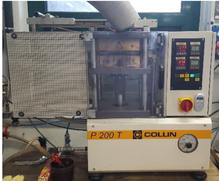
Fig. 84 – Platen press: the fusion process at 275°C
