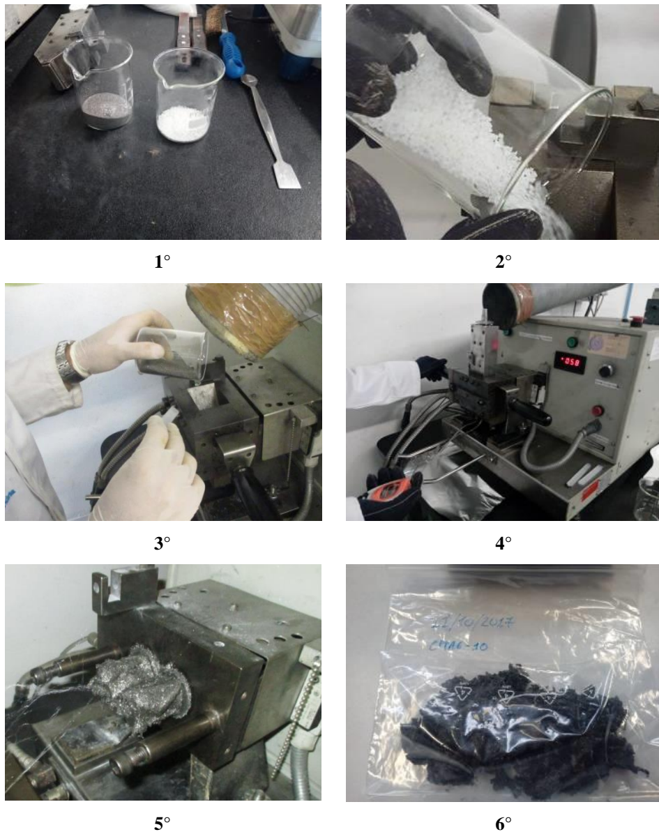
Fig. 31 – Stages of composite production using the dedicated plastic mixer: 1° choice of magnetic and polymeric correct quantities, 2° insert of polymeric binder in pellet form (PA6), 3° insert of magnetic powder, 4° mixed in brabender, 5° extraction of agglomerate material and 6° final compound shape
