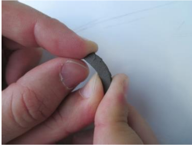
Fig. 60 – Magnetized sample of flexible magnet adopted in flux barriers
