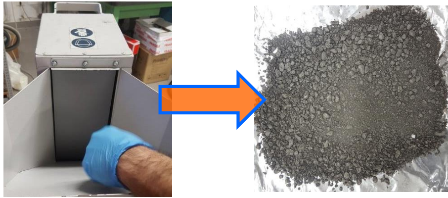
Fig. 32 – Grinding of produced composite with the aim to make the magnetic powder useful for the molding process
