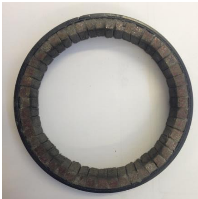
Fig. 145 – Final rotor geometry with NdFeB Halbach Bonded magnets
