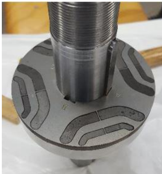
Fig. 101 - The insertion of the magnets in the flux barriers
