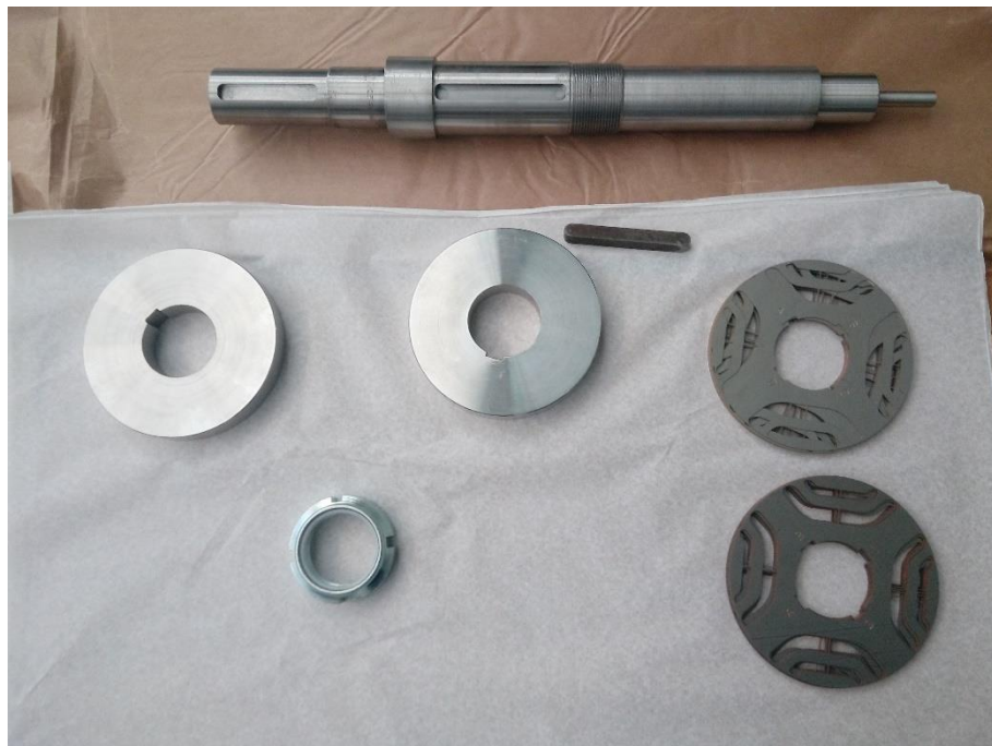
Fig. 98 – The main components of the rotor
