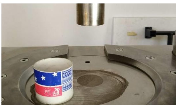
Fig. 27 - Compression process with the hydraulic press using different pressure levels
