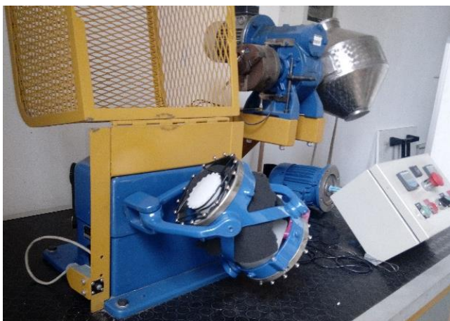
Fig. 26 – Automatic mixing process with turbula
