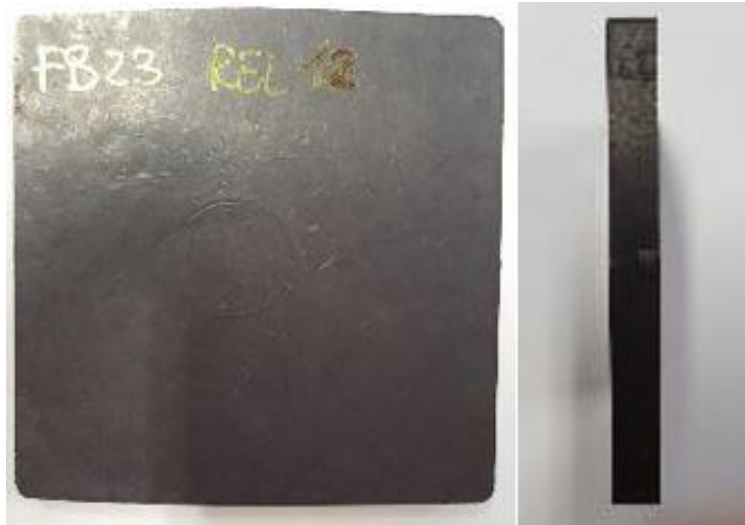
Fig. 91 - The molded sample of FB23 Ferrite Bonded magnets
