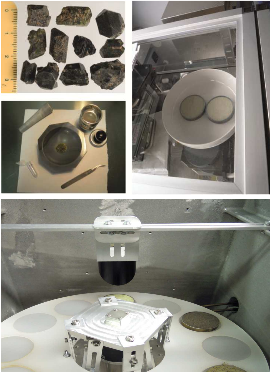
Figure 3.1. Sample preparation and vacuum chamber at PEL. a) Crystals of pyroxenes labeled DiMDCV. b) Grinding of crystals. c) Cups of samples in dryer chamber. d) Within the vacuum chamber, the cups are placed on a carousel.
