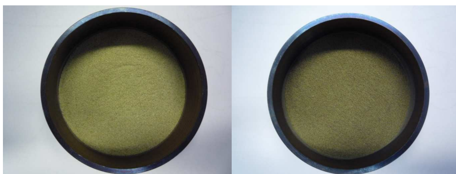
Figure 3.3. Unheated samples of diopside (DiMDCV at 0-125 \mu\text{m} , left side) and hedenbergite (HeE0125 at 0-125 \mu\text{m} , right side) prepared for the TIR vacuum chamber (see the text).
