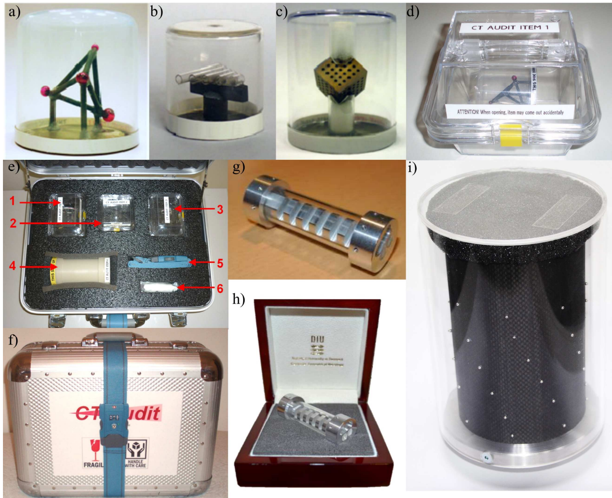
Figure 99. Examples of packaging of reference standards: a) tetrahedron in a sealed box [7], b) pan flute in a sealed box [7], c) calotte cube in a sealed box [7], d) tetrahedron in a membrane box [7], e) open suitcase with reference standards used for CT Audit [7], f) closed and secured CT Audit suitcase [7], g) multi-material assembly of a step gauge sealed in a glass tube used in [65], h) protective box for the step gauge for INTERAQCT comparison on assemblies [65], i) protected reference standard for CT instrument geometry calibration proposed in this Ph.D. thesis.
