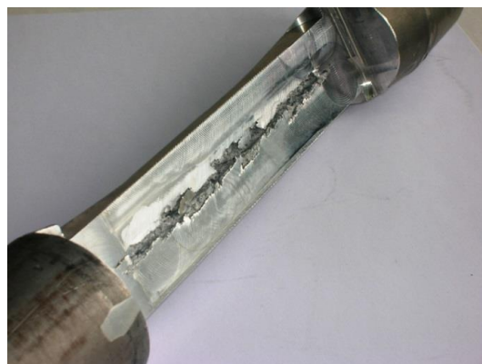
Figure 4. 3 – Axial cracking resulting from cross wedge rolling at 510^{\circ}\text{C} .
