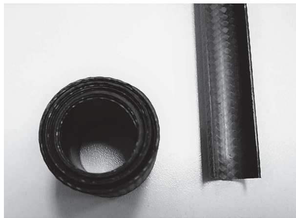
Figure 3.3: Photo of the booms in coiled and deployed configurations.
