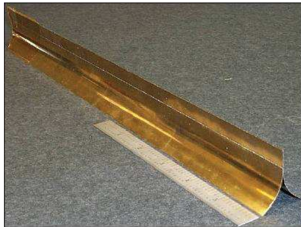
Figure 1.8: TRAC boom. Image credit: NASA
