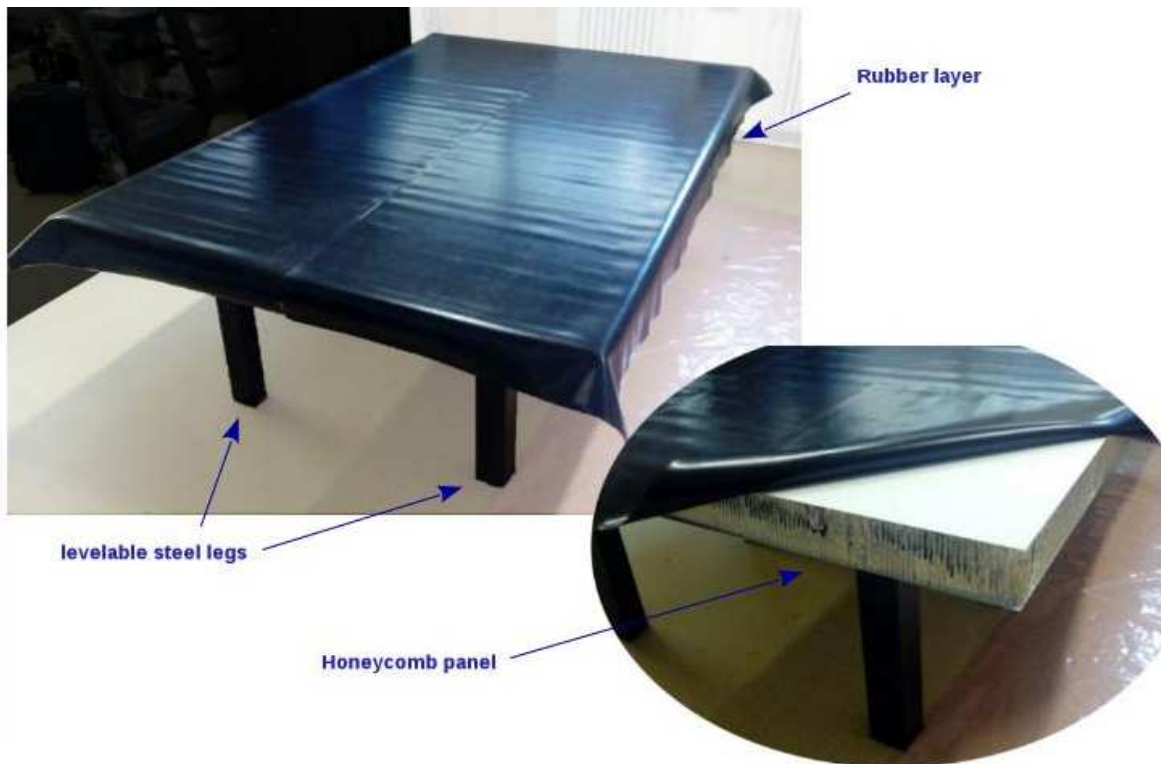
Figure 2.12: Test table with levelable steel legs, rubber layer and honeycomb panel. The glass sheet is not shown in the picture
