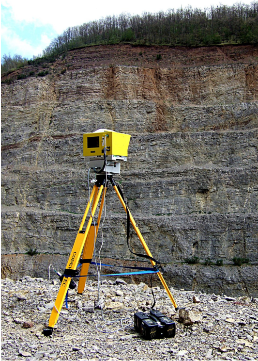
Figure 1.1: OPTECH ILRIS 3D terrestrial laser scanner during scanning.
