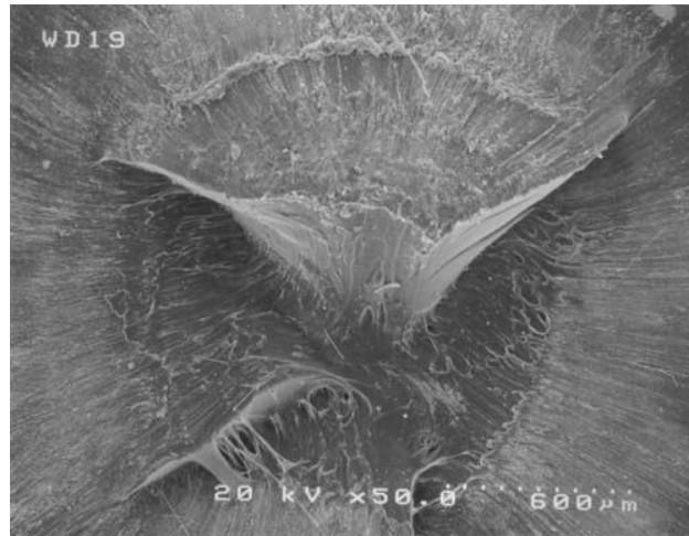
Figure 3.8 Scanning electron micrograph of healed EMAA ionomer following puncture with 4.5 mm diameter projectile [38].
