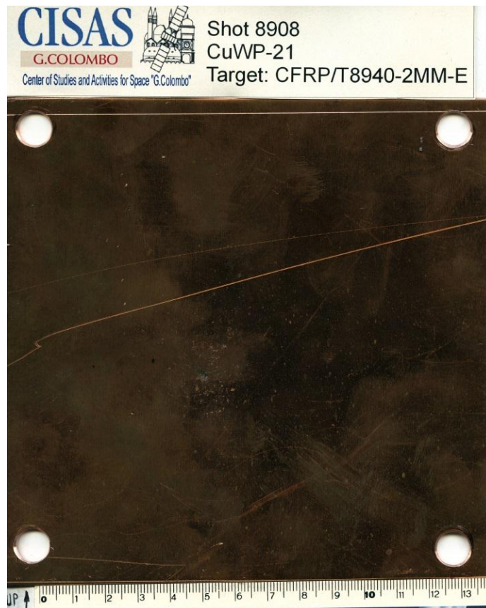
Figure 4.18 Witness plate after test 8908. A black crater is visible on the WP.
