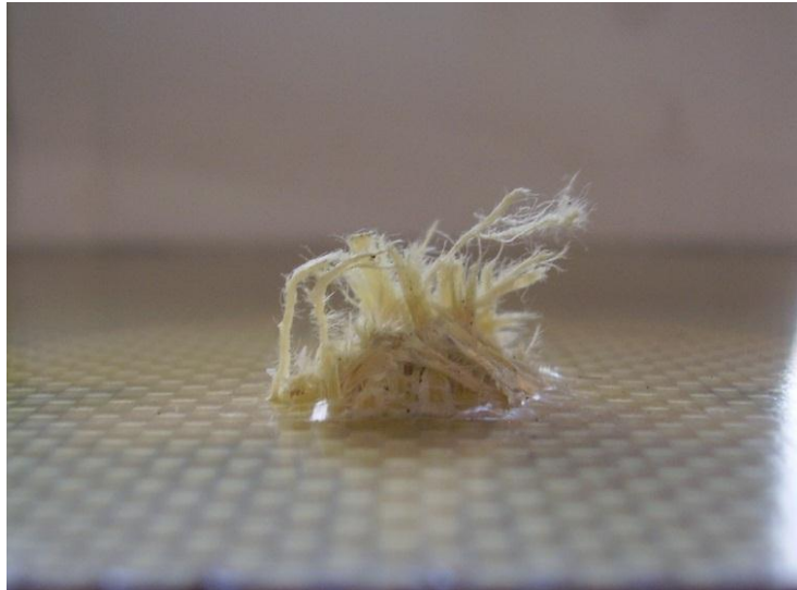
Figure 4.43 Aramid fibres sticking out normally from the panel C surface after impact.
