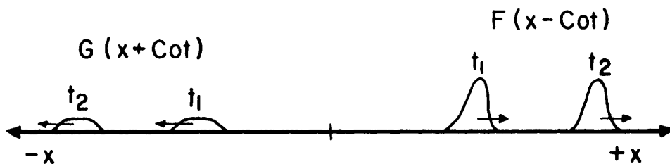
Figure 2.2 General solution for wave equation in uniaxial stress [5].
