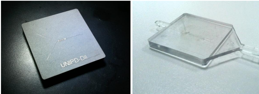
Figure 1.3: Example of microfluidic mixer obtained through micro injection moulding. Mould insert (left) and moulded part (right).
