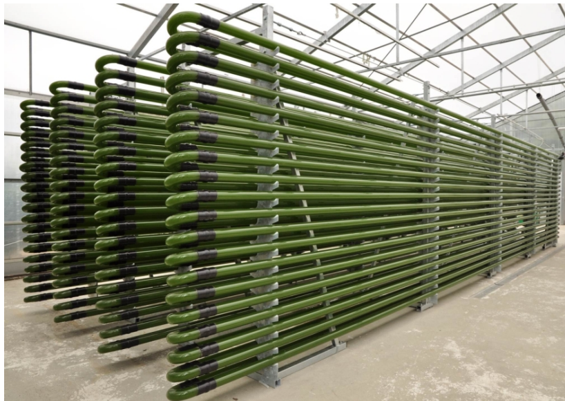
Figure 1.2: Tubular photobioreactor. (Foto: IGV Biotech)
