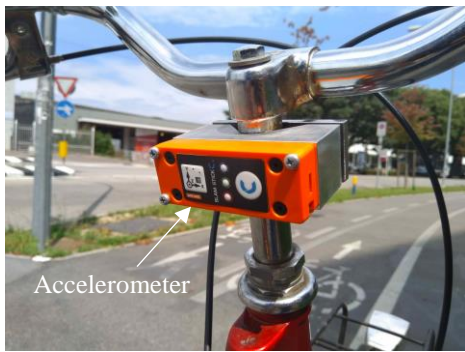
Fig. 1. Accelerometer mounted on the steerer tube.
