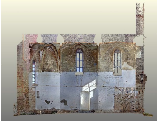
Fig. 3 Orthophoto Section South. Laser Scan Survey. Solvotek.
