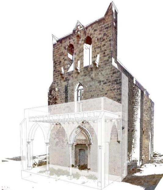
Fig. 9 St. Anne, 3D model overlapping with the point cloud. Reconstruction of the west porch.
