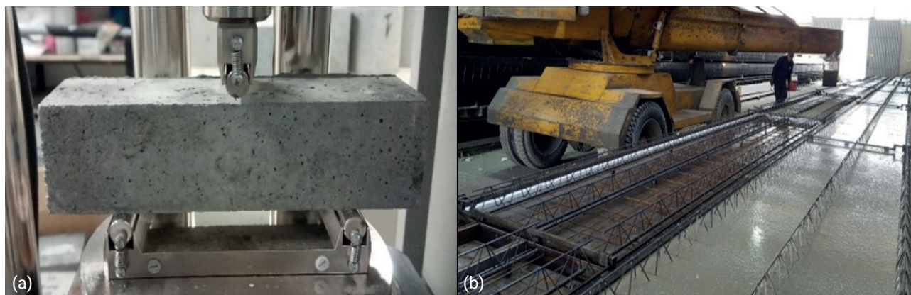
FIGURE 9: Building materials with glass from PV-panels: mechanical test on mortar (a) and industrial production of concrete (b).
