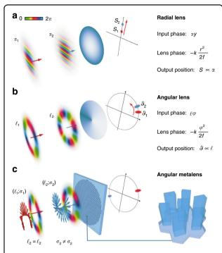
**Fig. 1 Working principle of the angular lens. a** A radial-quadratic phase focuses different linear phase gradients onto distinct axial positions. **b** An azimuthal-quadratic phase performs an analogous operation on orbital angular momentum (OAM) beams, mapping different azimuthal phase gradients onto distinct angular positions. **c** Its implementation in a metasurface form enables the combined measurement of polarization (spin *σ*) and OAM
